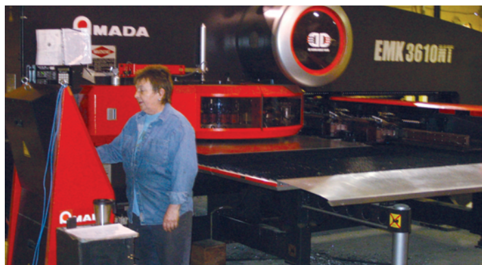
Installing an Amada EMK 3610NT turret punch press has provided Ritz Technologies with a number of benefits including increased production capacity and opened up new opportunities for business.
